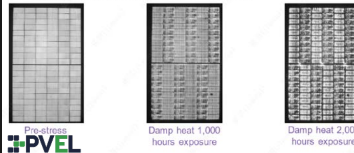
Figure 14: Example of damp heat testing exposure from the laboratory for TOPCon modules where cell degraded by 67.5% after 2,000 hours of exposure
