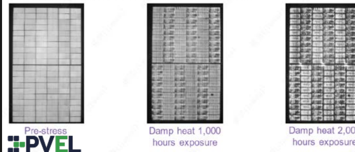
Figure 14: Example of damp heat testing exposure from the laboratory for TOPCon module where cell degraded by 67.5% after 2,000 hours of exposure
